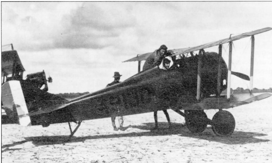
A "Tommy Morse Scout" powered by an 80-horsepower LeRhone engine, was photographed at Marine Flying Field, Miami, Florida, in 1915. Because of the Tommy's success as a trainer, it became one of the most popular single-seaters built in America.
